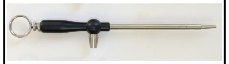
**Pro Series Pull Ring Drain Tubes**<sup>TM</sup> feature precision machined light weight high performance black Delrin body with a Precision Stainless Pull Ring and Stainless Steel Tube. Stainless Components resist corrosion and will not chip or corrode. Four precision machined slots provide for increased flow. Easily disassembled for cleaning.
