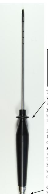
Our 3/16" Diameter Trocars feature stainless steel tubing and fittings, high performance light weight Delrin hand grip, and a precision hardened trocar point. All trocars come with a easy to remove safety cap for the point.
