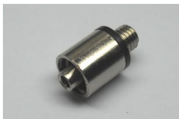
Part#: ADPR1045 Luer Adapter to 12 -32 Male Thread Includes 1 ADPR9352 Leather Washer
