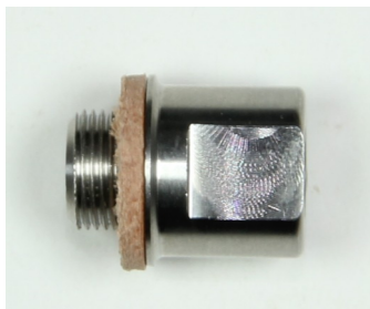
Part#: ADPR9261 Stainless Steel - Valve Handle To Arterial Tube Adapter (5/16-36 male thread to 12/32 female thread)
